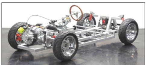
aluminum wheels and a 12-volt electrical system with electric start. The body is composite glass reinforced plastic. Curb weight is 214 lbs. The standard model is claimed in the website to be able to top 44 mph and owner-tuned versions are evidently
