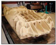
King Cobra plywood buck used to construct a replacement body during a recent restoration.
